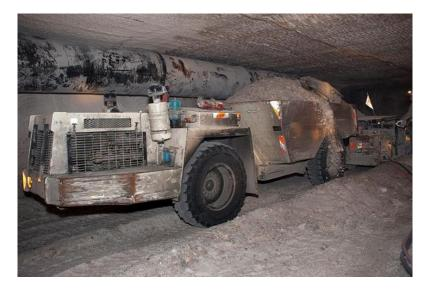
The EIMCO Model 985, 15 ton haul truck is a diesel powered vehicle used to haul salt from the mine. This is an aged piece of equipment, approximately 29 years old.
